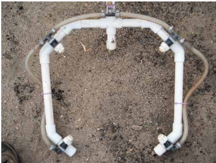
Fig. 5. Close-up of the business end of a home-built wand sprayer constructed using PVC tubing and fittings. Use a large nozzle and reduced spray pressure in order to eliminate drift to fruit or foliage. The butt of the wand rests on the ground and 4 nozzles apply the bifenthrin all around the trunk from a single entry into the tree. The opening of the U-shaped device must be wide enough to accommodate the largest trunk.
